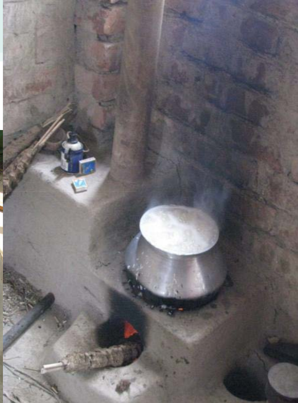
Right: Bondhu chula; the current model of improved stove most widely disseminated in Bangladesh. Built-in place chimney stove.
