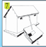
7 Finally fix the delivery pipe from the gutter to the cistern to have a complete rainwater harvesting cistern.
