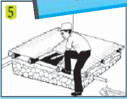
5 Make a cover for the pit by using iron sheets.
