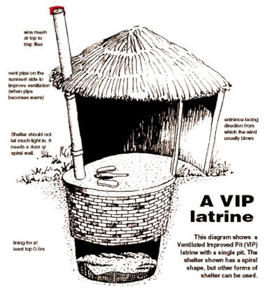
the principle that flies are attracted to light. To a fly in the pit, the squat hole will not be brightly illuminated so it will try to leave by going up the vent towards the sunlight shining down into the pit. The mesh will stop it escaping and it will eventually die.
