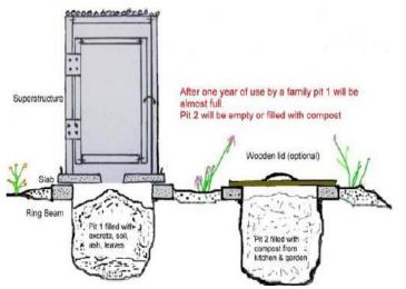
• Can use in conditions that prohibit deep pits, e.g., hard to excavate rock, collapsible sand or high water tables
