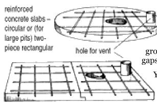
The size of the slab can be the same size as the outer lining if this is built of brick. If the lining is made from an oil drum or basketwork it needs to be slightly larger so that at least 200mm of the slab rests on the ground all round the pit. There should not be any gaps under the slab to let flies or smells leave the pit.
