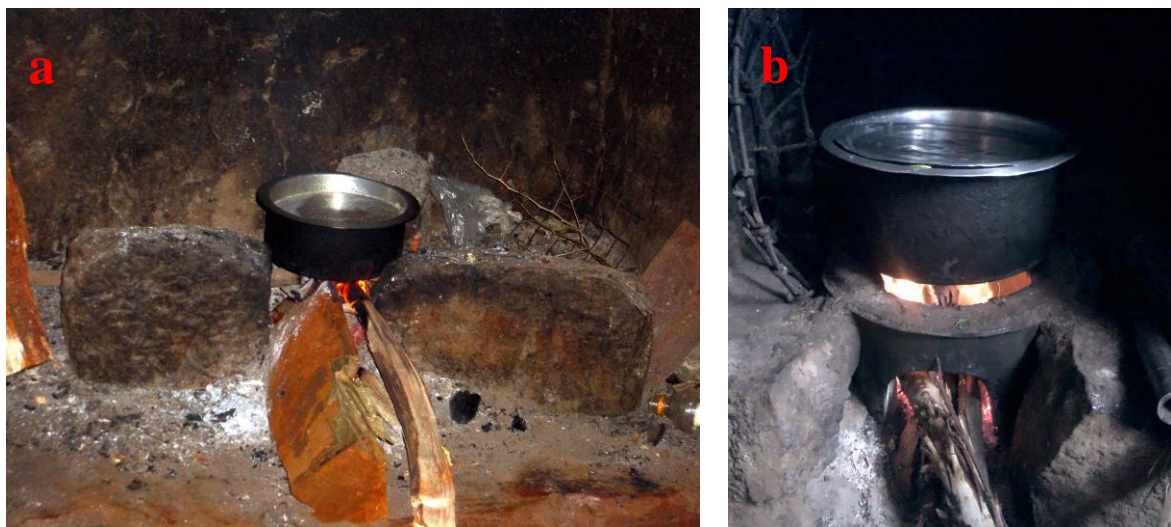
Figure 2: Stove photos: (a) three-stone fire, (b) Jiko Kisasa, (c-e) other baseline stoves, and (f) Jiko Poa.
