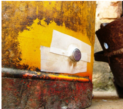
Figure 3: Stove Use Monitoring System (SUMS)
