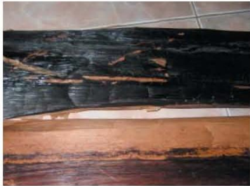
Waterproof inside layer of 2 banana fiber pieces
