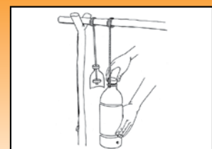
Loosen lid to allow water flow and tighten lid to stop water flow.
