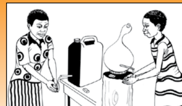
To start water flow, remove container lid or plug. To stop water flow, put tight the container lid.
