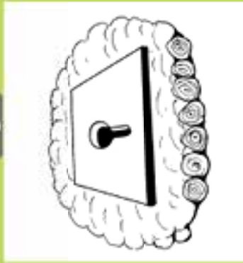
Cover the logs or wood with mud, leaving a squat hole of about 12.5x25 cm. If possible, install a SanPlat to make the latrine easy to clean and look modern.
