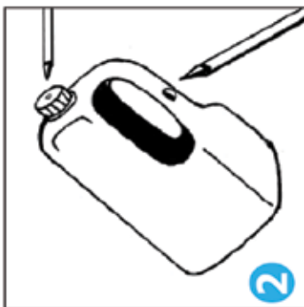
Using a nail, punch a hole on the lid for the pedestal string and at the jerry can handle for the dripping water.
